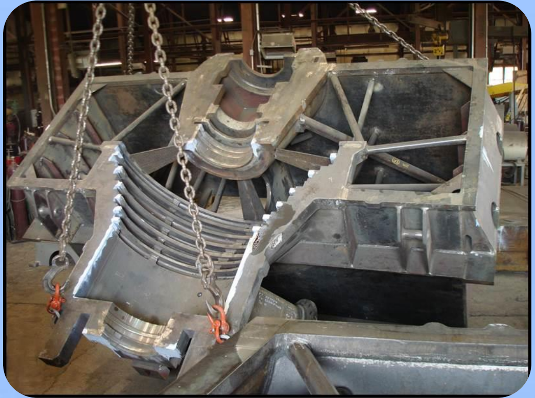
Fabricated Steam Turbine Casing Section (Replacement for a Cast Casing)
