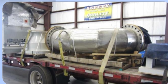
Fabricated Process Pipe Spools with Mitred Elbows and Internal Turning Vanes
